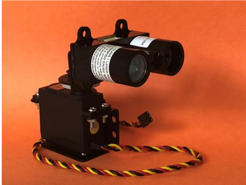
Figure 18: Test setup of 180° LIDAR performed by the team
